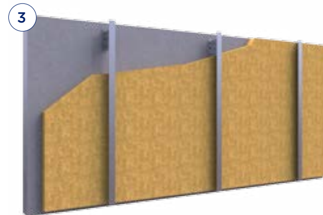
Fixing the "L" shaped profiles
