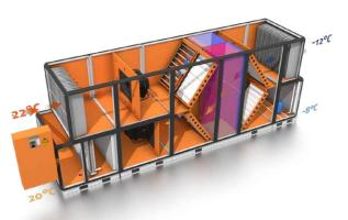
The unit contains two heat storage packets with highly sensitive accumulator mass, through which the outside and return air are transported alternately. The accumulator mass is able to capture heat from a warm air flow very rapidly and transferring this just as rapidly to the cold air flow.
