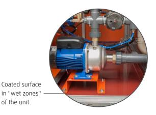
CNC-bended pipework for all compression cooling plants. That means significantly less solder connections and thus fewer weak
