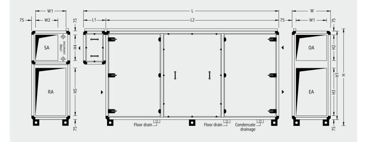
Unit feet 100 mm Optionally: adjustable feet from 100 to 120 mm
