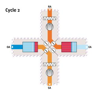
The unit contains two heat storage packets with highly sensitive accumulator mass, through which the outside and return air are transported alternately. The accumulator mass is capable of capturing heat from a warm air flow very rapidly and transferring this just as rapidly to the cold air flow.
