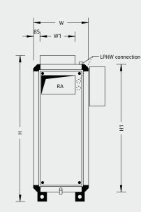
Unit feet 100 mm Optional: adjustable feet from 100 to 120 mm
