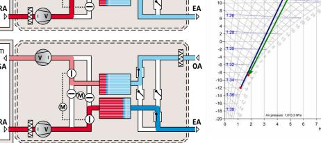
The unit contains two heat storage packets with highly sensitive accumulator mass, through which the outside and return air are transported alternately. The accumulator mass is able to capture heat from a warm air flow very rapidly and transferring this just as rapidly to the cold air flow.
